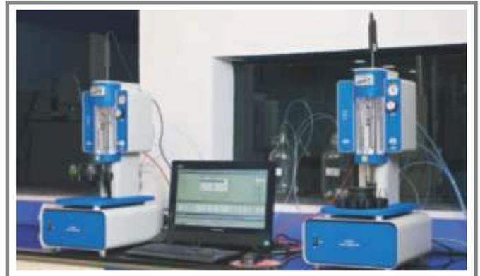
Canon Auto Viscometer to Test Viscosity of Industrial & Automotive Lubricants
