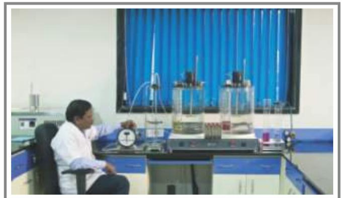
Auto Foaming Apparatus to Test Foaming Characteristic of Industrial & Automotive Lubricants
