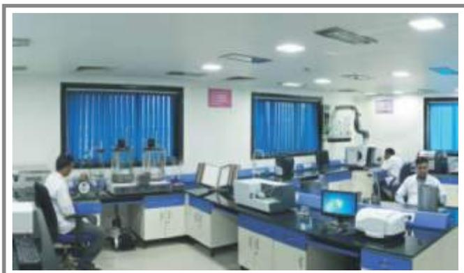
R & D Analytical Lab – II having FTIR for carbon type analysis, TNTS for Nitrogen and sulphur analysis, Foaming Tester, ICP for Elemental Analysis
