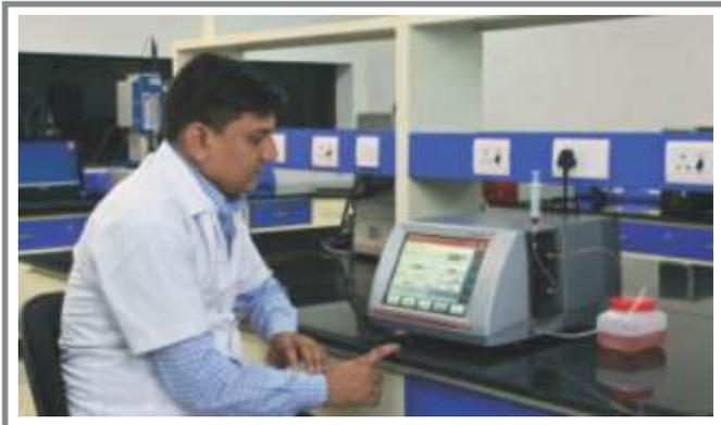
Auto Viscometer to test Viscosity & Density of Industrial & Automotive Lubricants
